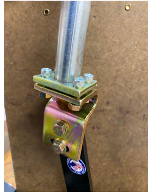
48" RELOCATED HANDLE PIVOT BRACKET VIEWED FROM DECK OPENING
